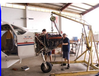
Engine installation on a GA8
